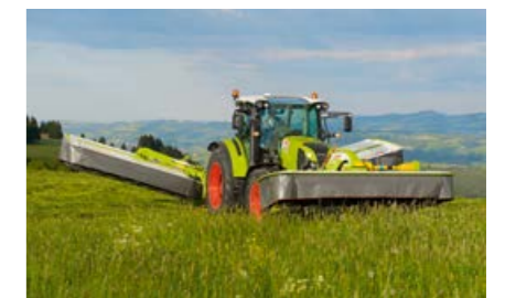
Compact suspension at the front linkage gives the mower generous ground clearance at headlands.
