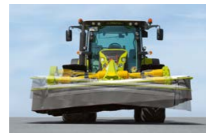
Freely pivoting mount for adaptation across the direction of travel.
