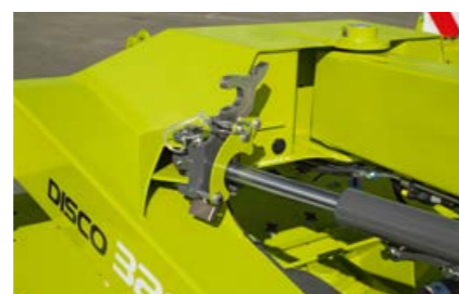
Flexible: optional tool-free drawbar adjustment for rapid adaptation to different tractors.
