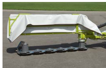
The protective covers fold well up, for easy access to all maintenance points.
